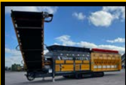
BARFORD T722R TRACKED TROMMEL WITH RADIAL FINES CONVEYOR
